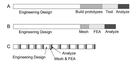
**Figure 2.13.** Comparison between different development strategies in foremost the automotive industry, A: old-fashioned, B: contemporary, and C: modern (Holmdahl 2003)
