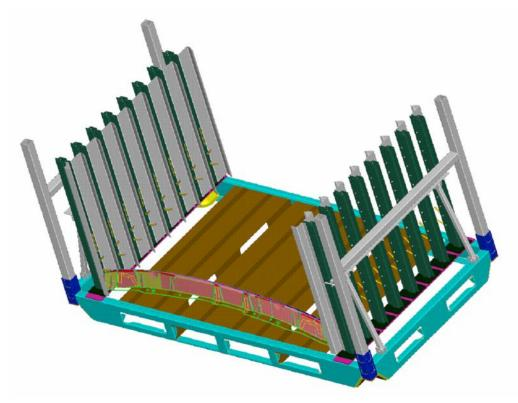
Figure 5.4. The Weibulls' torpedo beam rack with one torpedo beam in place
