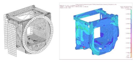
Figure 6.15. A camera house analyzed with FEA through the use of COD
